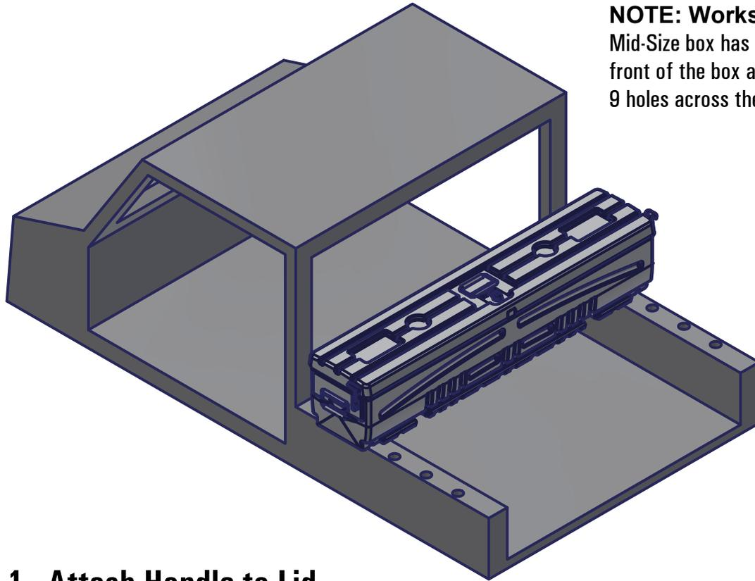
**NOTE: Works on Mid-size box only.** Mid-Size box has 7 holes across the front of the box and the Full-Size box has 9 holes across the front of the box.
